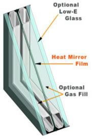
Coated Heat Mirror films are often used in conjunction with low-e glass, taking advantage of the benefits of both film-based coatings and glass based technologies. Inert gases, such as argon or krypton, are added to create Heat Mirror insulating glass units with industry leading performance. Outstanding winter insulation and superior solar control provide year-round savings and enhanced comfort.
